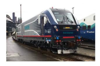
**Electric Loco** w/Diesel or Battery **Power Tender**
